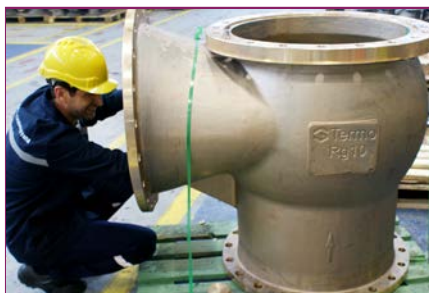
Gedik Advanced Casting Technologies has casted, DN 600 Angle Glob Valve Manufactured by the Gedik Termo Valve
